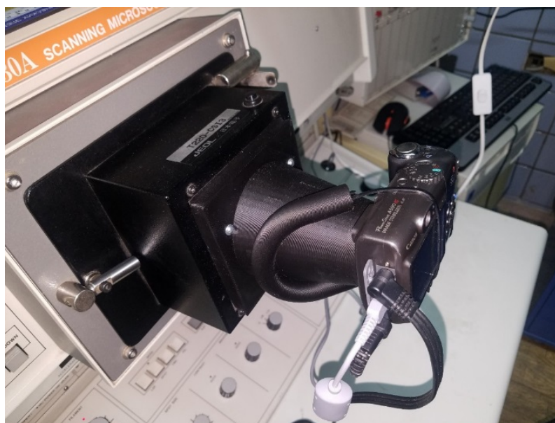
Fig. 2. Canon A590IS fixation on the 3D printable adapter for optical registration tract from the CRT
